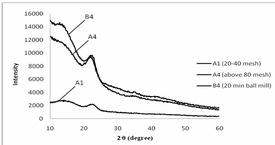
Fig. 5. XRD spectra: (A1) 20-40 mesh, (A4) above 80 mesh and (B4) 20 min ball mill.
